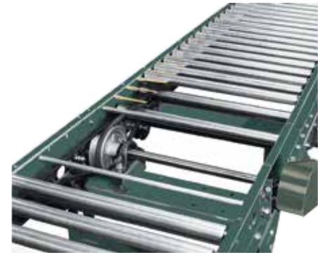
Conveyor sections are easily coupled together at either end to make up to 100 ft. long units. Drive is usually located near center of conveyor.
